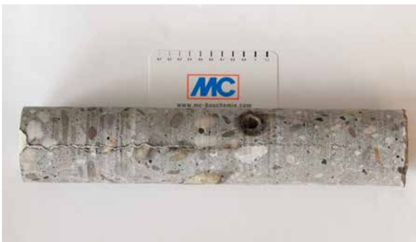
This section through an injected component clearly shows the depth of penetration achieved with MC-Injekt 2133 flex through even the finest of hairline cracks.
