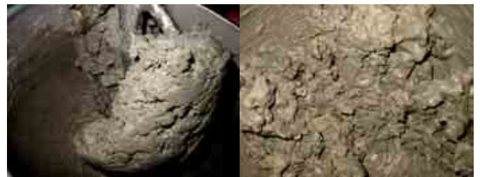
Figure 6: clay behavior without and with anti-clay polymer
