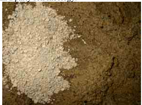
Figure 7: comparison of original pure dry porous soil and as homogeneous paste after mixing with foam and polymer
