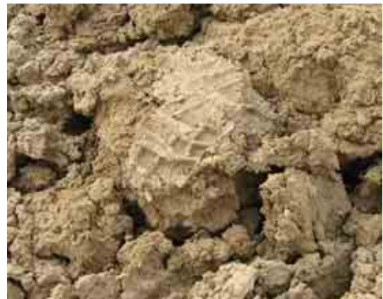
Figure 14: soft but not adhesive soil after excavation
