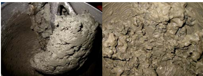
Figure 3: clay behaviour without and with anti-clay polymer
