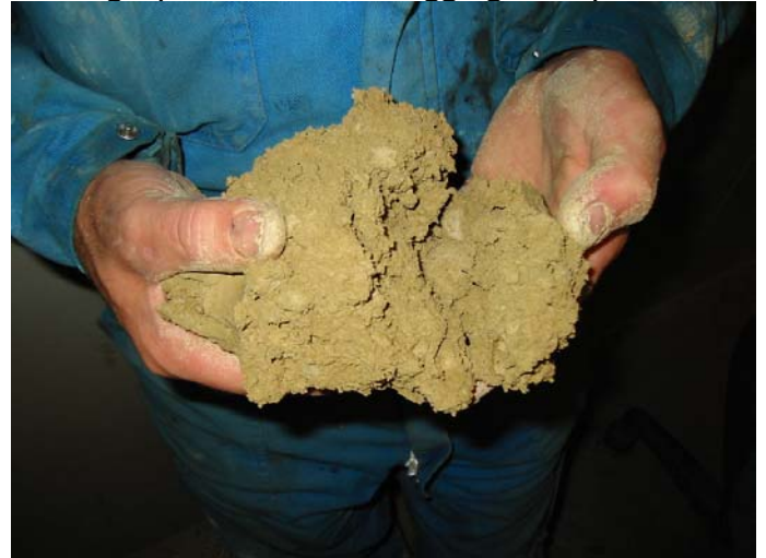
Figure 12: plastic & non clogging excavated soil
