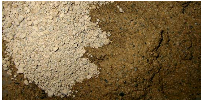
Figure 4: comparison of original pure dry porous soil and as homogeneous paste after mixing with foam and polymer
