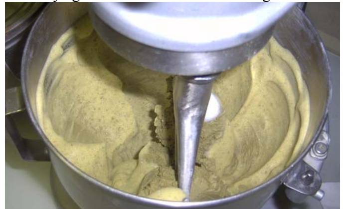
Figure 9: correct EPB conditioning in the laboratory
