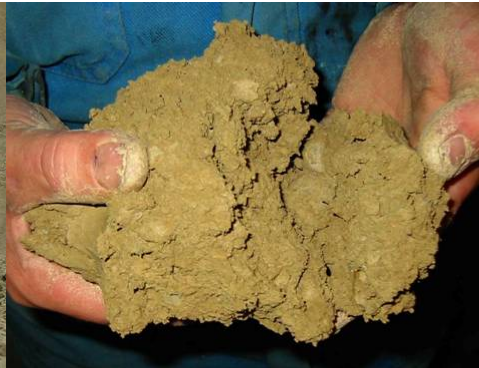
Homogeneous & plastic soil with MEYCO SLF 30 and Rheosoil 211
