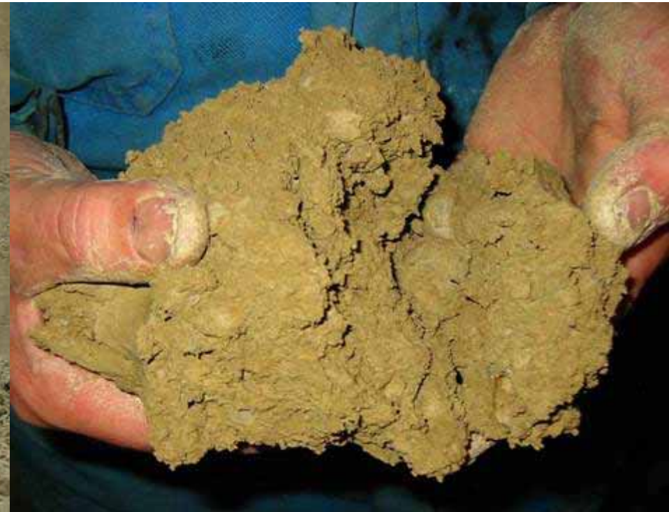
homogeneous & plastic soil with Foam and RHEOSOIL
