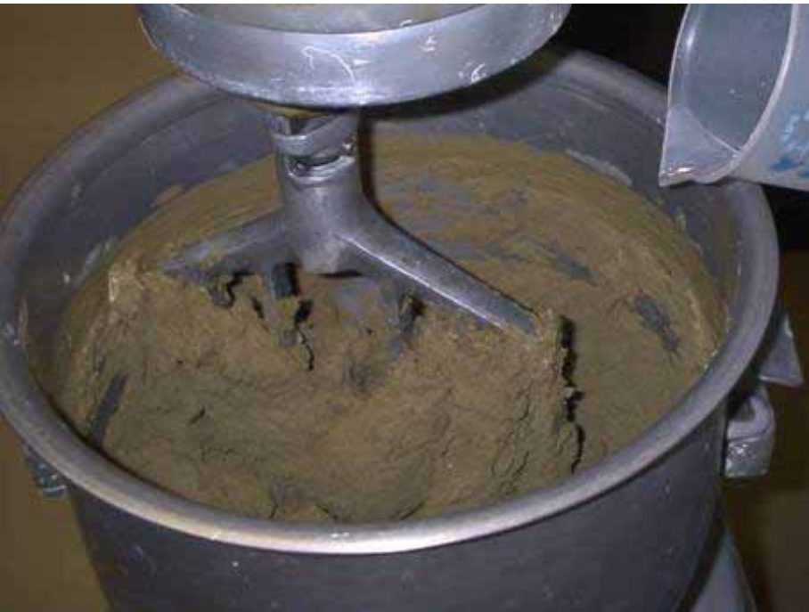
Addition of water and standard foam
