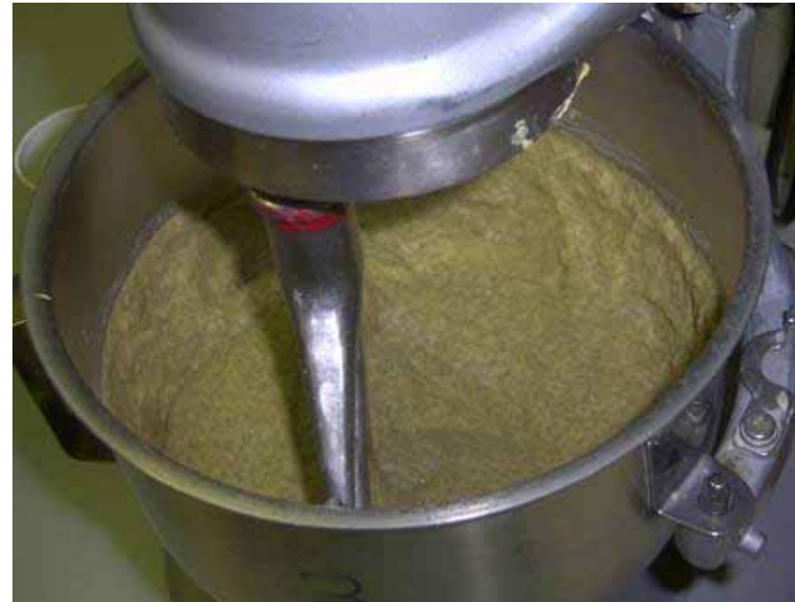
Addition of water, Foam and RHEOSOIL anti-clay-agent
