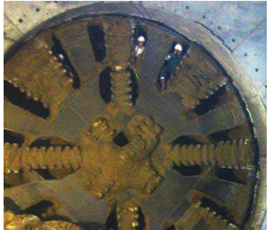
plastic mode & full chamber with RHEOSOIL®
