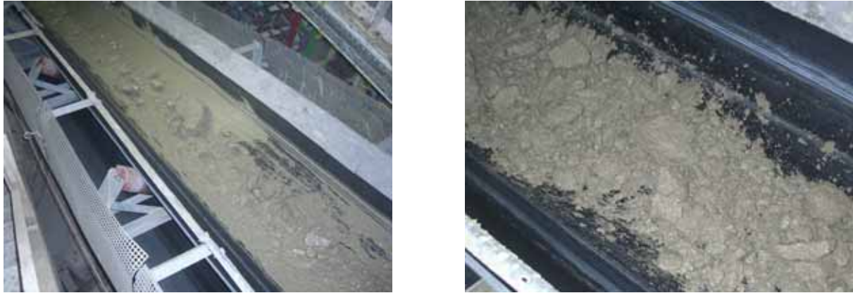
Figure 10: Rock treated with water spray (left) and with ABR5 anti-abrasion additive (right)
