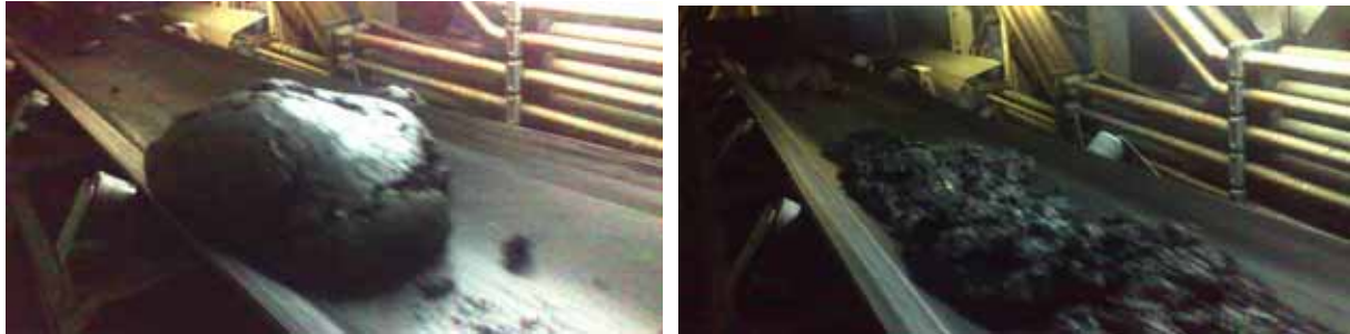
Figure 5: Clay balls on the belt without and with Rheosoil143
