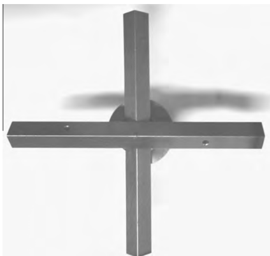
Fig. 2. The SGAT drilling tool. The test pieces have 1 × 1 cm cross-section, and the holes on the lower steel bar is the nozzles for soil conditioning additives.
