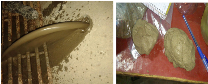
Fig. 13. Running silty sand with no cohesion. Increased cohesion and decreased permeability with the use of polymer.
