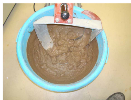
Fig. 15. Cochem shale (borehole sample) and conditioned soil with anti clay agent and fine filler suspension.
