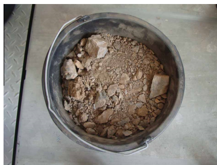
Fig. 15. Cochem shale (borehole sample) and conditioned soil with anti clay agent and fine filler suspension.
