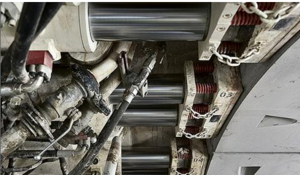
Fig. 14 Standard Herrenknecht 2k injection system, invert view
