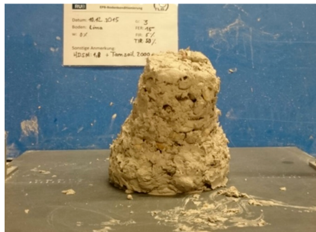
Figure 6. Result of the Slump Test No. 1 with w=0\% , density of the slurry 1,8 \text{ g/cm}^3 , ASIR=50%, c_f=3\% , FER=15 and FIR=15%. The measured Slump was 12 cm.
