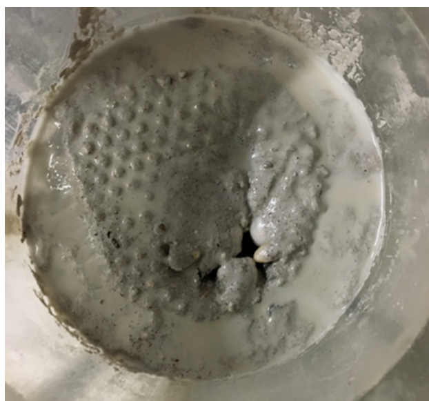
Figure 10. Flow out of the conditioning agents during the water permeability test.
