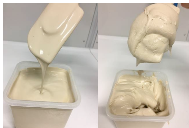
Figure 5. Production of artificial soil based on High Density Slurry and TamSoil 2000 CP (left: HDS with component A. Right: Slurry turned into Artificial Soil after adding component B)
