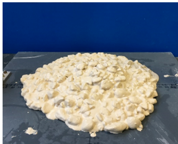
Figure 7. Result of the Slump Test No. 2 with w=5\% , density of the slurry 1,8 \text{ g/cm}^3 , ASIR=50%, c_f=3\% , FER=15 and FIR=15%. The measured Slump was 22,5 cm.
