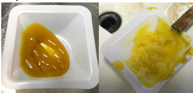
Figure 4. Water binding polymer TamSoil 1000CP (left) and the effect after adding water (right)
