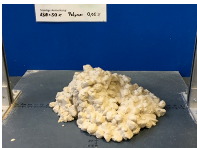
Figure 9. Result of the Slump Test No. 3 with w=5\% , density of the slurry 1,8 \text{ g/cm}^3 , ASIR=50%, c_f=3\% , FER=15, FIR=15% and PIR=0,05%. The measured Slump was 17,5 cm.
