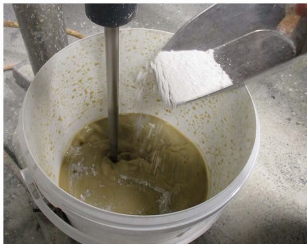
Figure 3. Production of a High Density Slurry by adding limestone powder into the bentonite suspension
