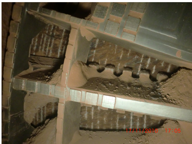
Picture 3: Cutterhead in hard rock conditions
