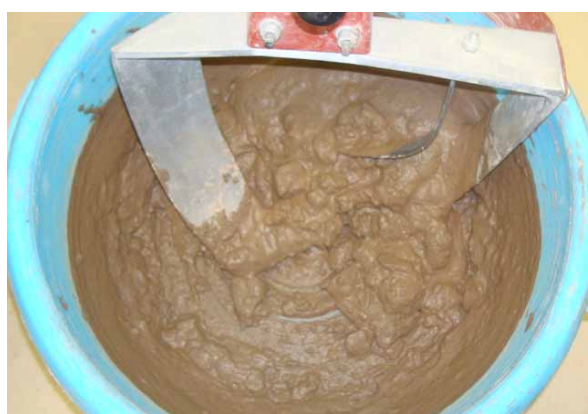
Picture 8: Cochem shale conditioned with foaming anti clay agent and additional fine filler suspension
