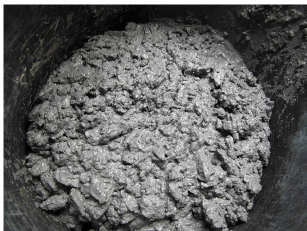
Picture 10: EPB like soil paste after conditioning process on the TBM
