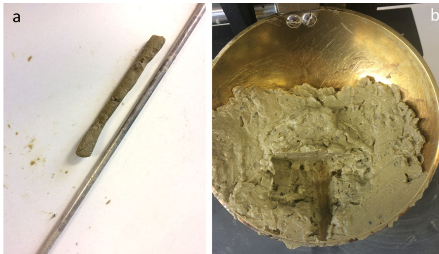
Fig. 7 Physical limitations of performing the plastic (a) and the liquid (b) limits on samples with coarser grains than the assumed threshold of the method (grains smaller than 0.425 mm). The
