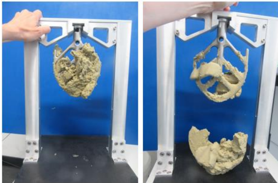
Figure 4. A.T.U.R. device designed to add a free fall drop to the beater with the soil stuck on it, after the first stage of mixing the soil with the HOBART machine. On the left, the beater before the drop and on the right, after the first drop, showing the partial release of the material.
